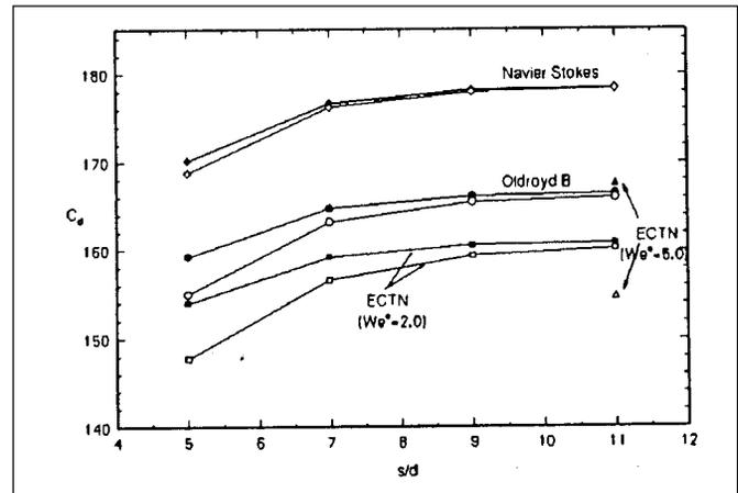
Fig. 3.1.2. Drag coefficient ( $C_d$ ) for a two-cylinder system; full symbols for the first cylinder and hollow for the second cylinder.
