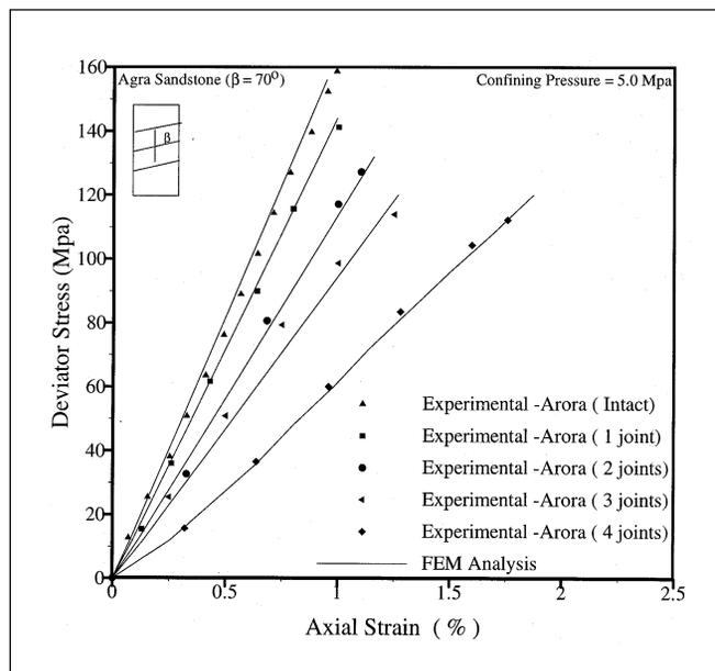
Fig. 3.4.2. Stress-strain plot for intact and multiple jointed specimen (experimental data after Arora, 1987).
