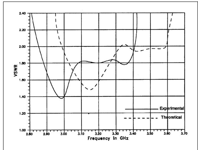
**Fig. 3.3.4.** Voltage Standing Wave Ratio comparison between experimental and the new model
