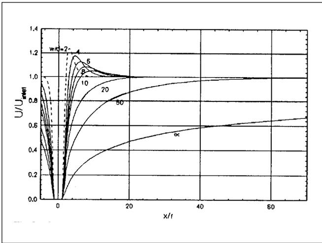
Fig. 3.2.1. Velocity along the wake for various  $w/d$  with  $De=5.95$ .
