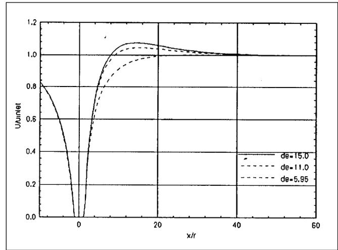
Fig. 3.2.2. Velocity along the wake for various  $De$  with  $w/d = 20$ .
