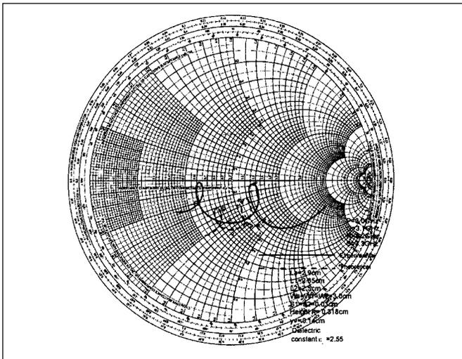
**Fig. 3.3.3.** Impedance comparison between experimental and the new model
