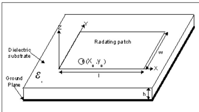
Fig. 3.3.2. Geometry of a gap-coupled patch antenna
