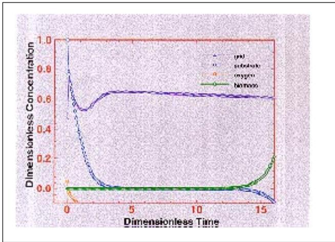
**Fig. 3.3.1.** Evolution of concentrations during remediation process computed using a finite difference moving grid method based on method of lines.
