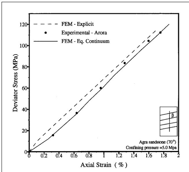
**Fig. 3.2.1.** Comparison of FEM results where joints in a multiply jointed specimen of Agra sandstone are explicitly represented and where they have been approximated through an equivalent continuum model; experimental results are also provided.
