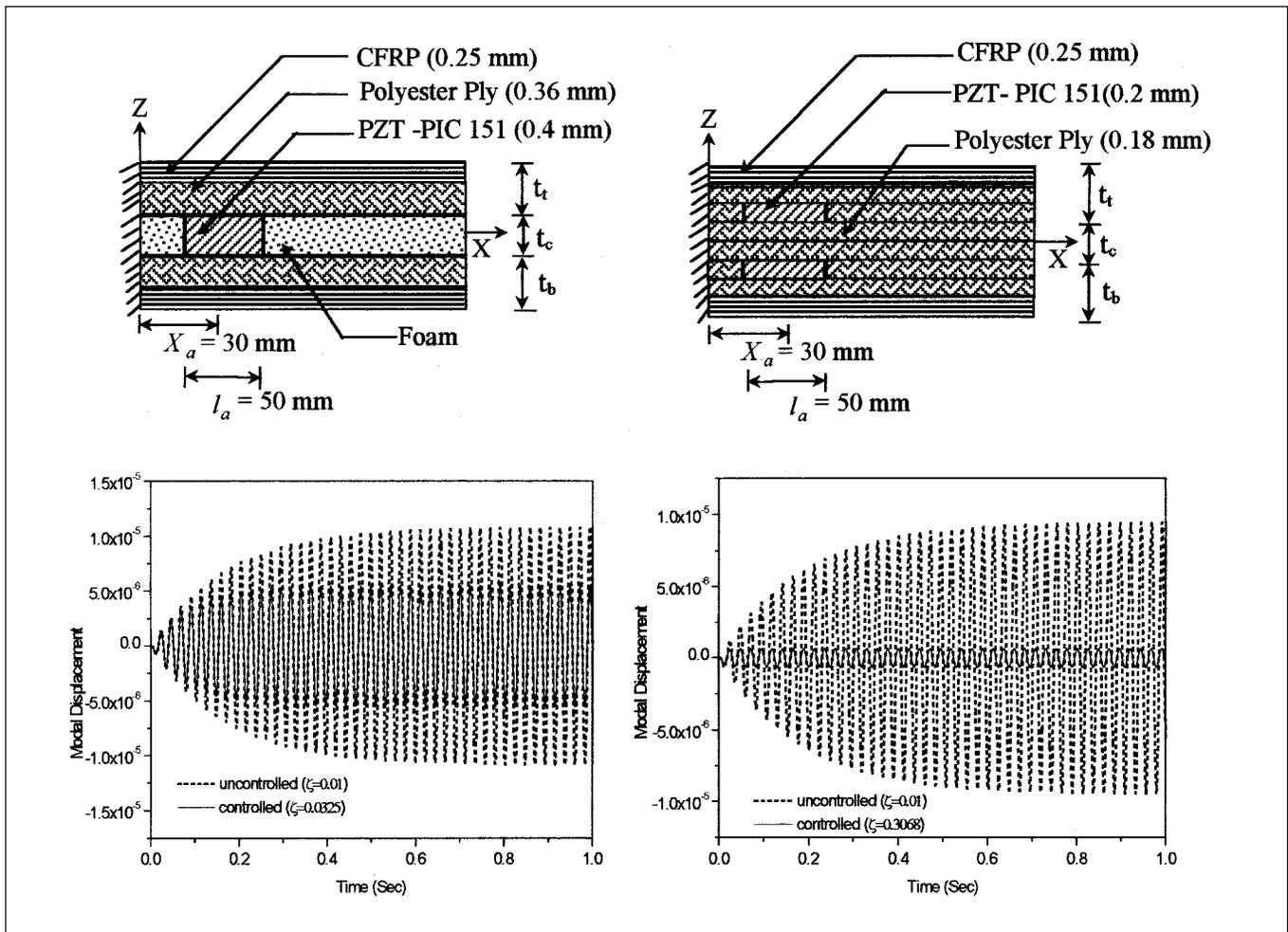
**Fig. 3.1.2.1.** Composite sandwich beams first mode control with shear actuation and extension-bending actuation (former is shown in the left panels and the latter in the right); top panels show the configurations and the bottom panels the establishment of control.
