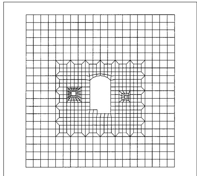
**Fig. 3.2.2.** Finite element mesh used for modelling a cavern and the surrounding rock.
