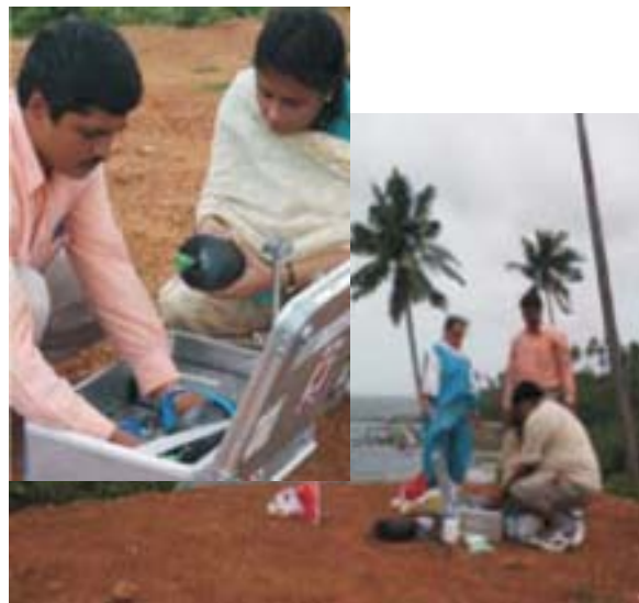
Figure 1.8 Air sampling at Port Blair using 1 lt glass flasks for collection of air.
