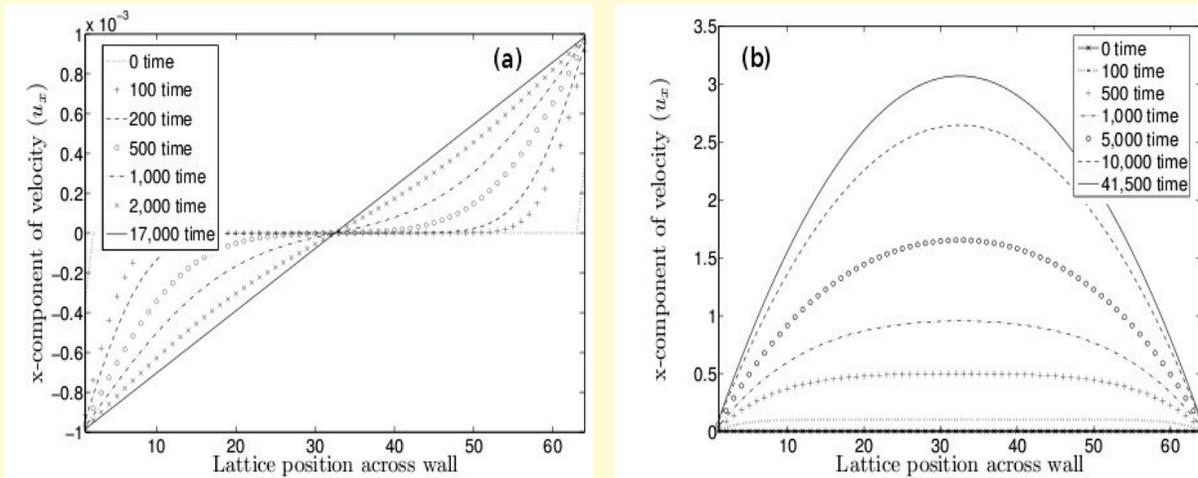
Figure 3.2 Velocity evolution of the fluid phase with time for (a) Couette flow and (b) Poiseuille flow
