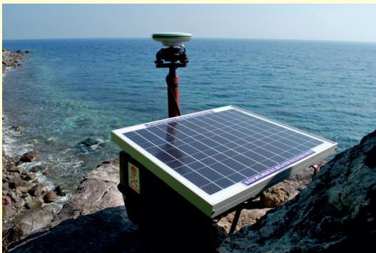
Figure 6.6 GNSS antenna mounted on the short drilled monument at the Narcondam Island.
