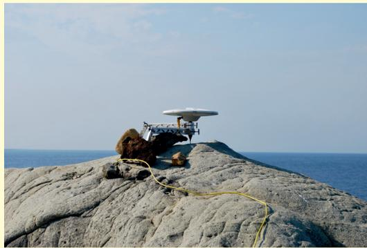
Figure 6.8 The campaign survey setup set ready at Burma Chad Island, west of North Andaman.
