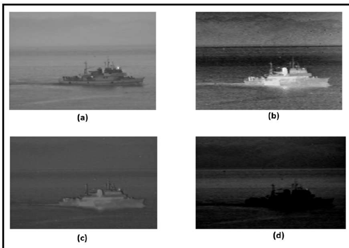
Figure 1.9: The images of “Ship” and the fused outcomes achieved by different algorithms. (a) VIS, (b) IR, (c) Fused Image using Bilateral Filtering Method, (d) Fused Image using Gaussian Filtering Method.
