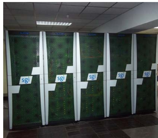
Figure 4.8 Altix ICE system with 2304 processing cores distributed over 192 nodes and 30 TB of parallel file system along with all associated hardware and software.
