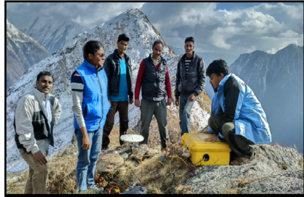
Figure 6.3 Campaign survey GPS set-up at Sukhi, Uttarakhand
