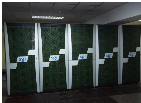
Figure 4.11 Altix ICE systems with 2304 processing cores distributed over 192 nodes and 30 TB of parallel file system along with all associated hardware and software.
