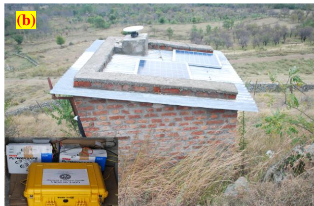
Figure 6.12 (a) Kashmir Valley CGNSS Network (b) CGNSS Station (Batpal) in Kashmir Valley (Insert shows instrument setup)
