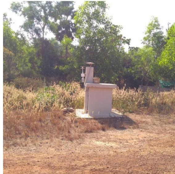
**Figure 5.6 CGNSS station with meteorological sensor established in Udupi, Karnataka**
