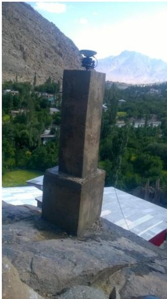
**Figure 5.5 CGNSS station established in Kargil, J&K**
