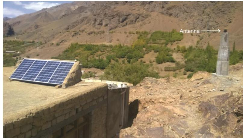
**Figure 5.4 CGNSS station established in Bhimbat, J &K**
