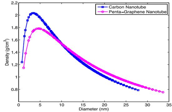
**Figure 6.3 Mass density comparison of Penta-Graphene nanotube with Carbon nanotube**
