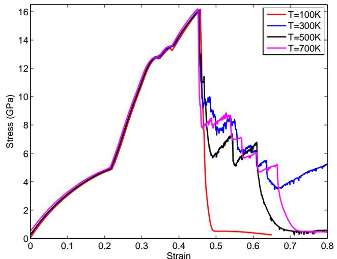
Figure 6.2 Stress-Strain Curve of Penta-Graphene nanowire
