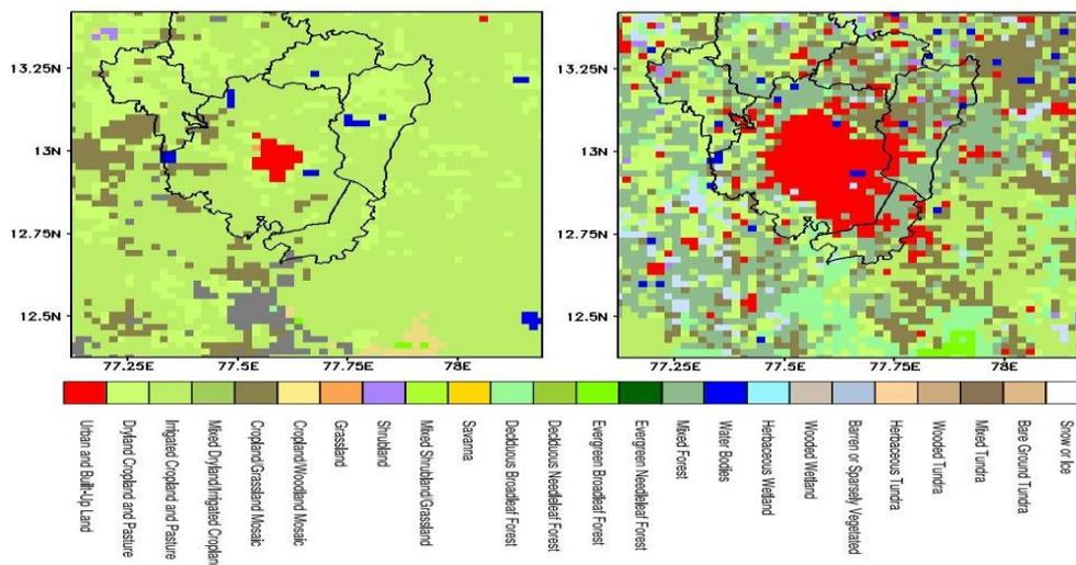
**Figure 2.4 High resolution land-use pattern over Bengaluru; USGS (left) and ISRO (right) used in WRF-UCM for rainfall simulation. A three-fold increase in urbanization over the central region of Bengaluru between 1992 and 2017 is evident in the right panel**
